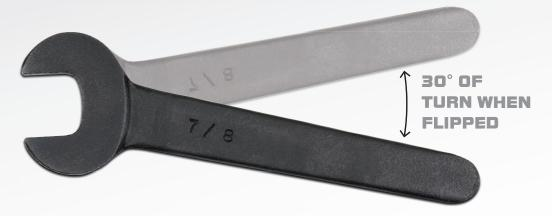
The check nut wrench tightens fasteners (sometimes called lock nuts or jam nuts) that lock other fasteners in place. The thin profile is used to squeeze into a tight space, or to rotate a fastener without moving the one next to it.
